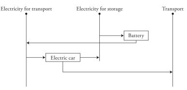
Figure 2: Electric Vehicle Modeling in ETEM
